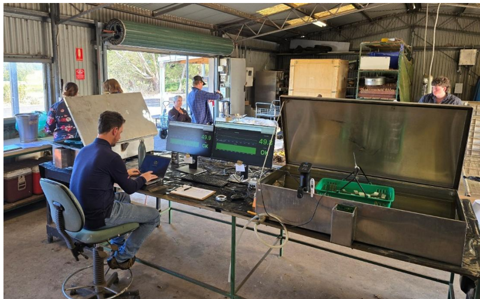
Hot water treatment set-up with multiple sensors logging temperature
