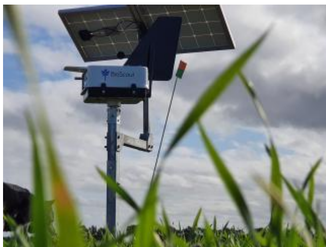
Image 19: BioScout's SporeScout unit in a wheat crop. Photo courtesy of: BioScout.
