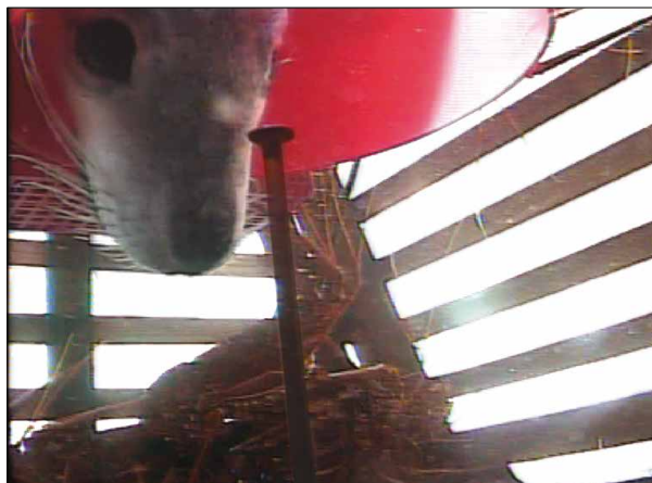
This internal SLED juts vertically from the pot's base so the sea lion can't get in.
