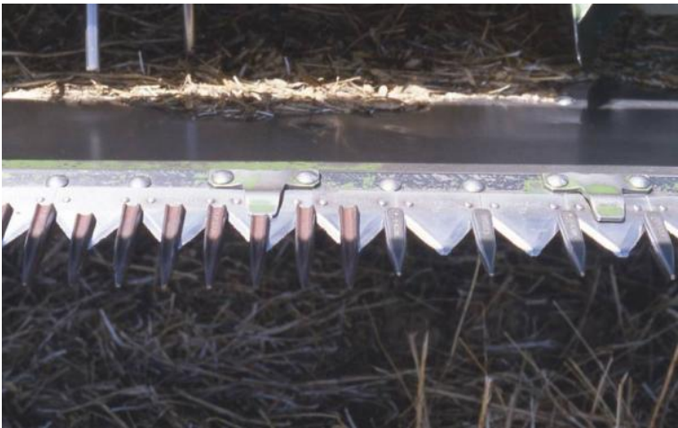
Figure 8. Four or double density (left) and 2 or single density knife guards (right)
