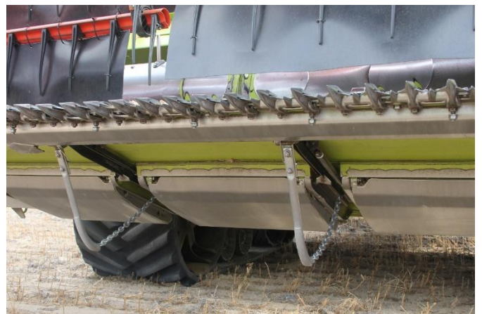
Figure 4. Claas Vario front with on-the-go knife extension
