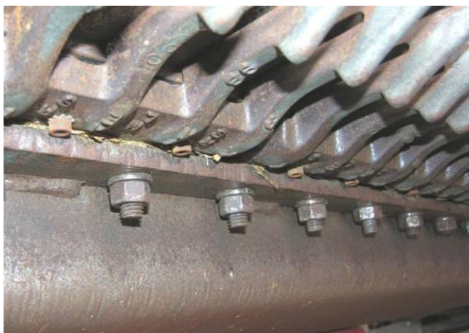
Figure 13. Raised knife guards on a Case 1040 belt front
