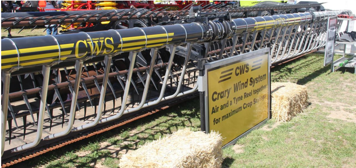
Figure 6. A Crary® air reel attached in front of a belt front with a tine reel
