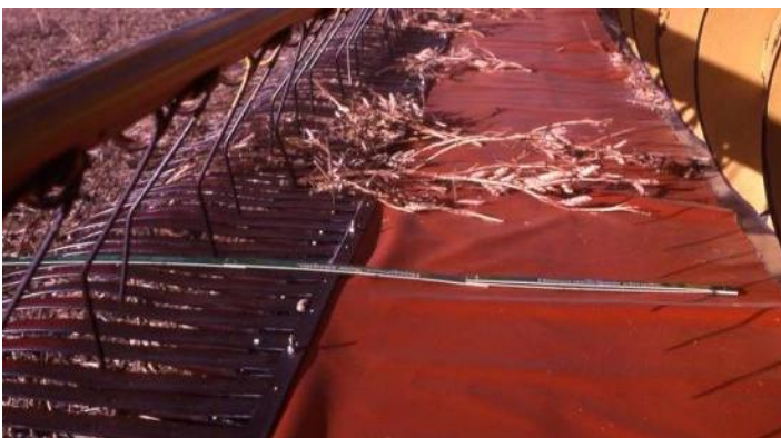
Figure 11. Vibra-mat® fitted to a knife
