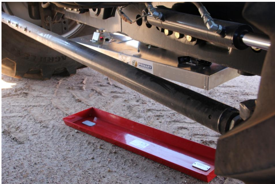
Figure 5. Example of a drop tray under the harvester rear axle to measure machine losses.
