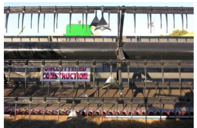
Figure 12. Paddle tines staggered around a tine reel.
