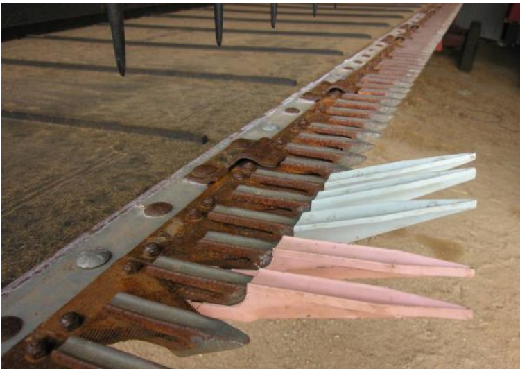
Figure 9. Straight and angled extension fingers on Primary Sales Australia knife guards
